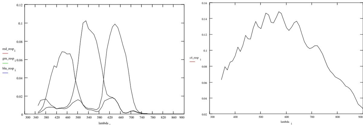
**Figure 6 Color and Monochrome Sensor Spectral Sensitivity**
