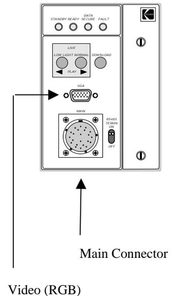
**Example of a Configuration (Same connection as the 16 mm film cameras, Photosonic 1PL)**
