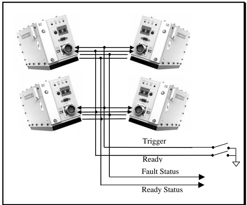
initialized and triggered. The Imager status can be monitored from a common set of lines that indicate each imager's state by their DC voltage.
