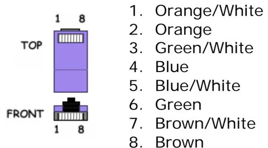
The wiring order for a straight-thru cable when viewing the RJ-45 connector from the topside of the connector (latch side down) is left to right. This cable is used between a computer and a hub or switch or between a standard hub/switch port and the uplink port of a cascaded hub/switch. Both ends of the cable are wired identically.
